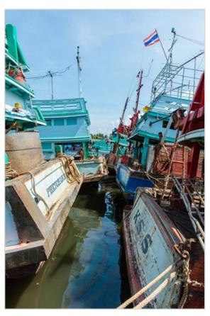
Trawler vessels in port. Note the red-brown doors on the back of some vessels, indicating otter board trawlers.
